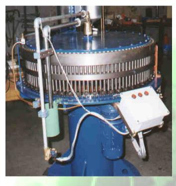
The cylinder casting machine is studied to produce lead cylinders.
