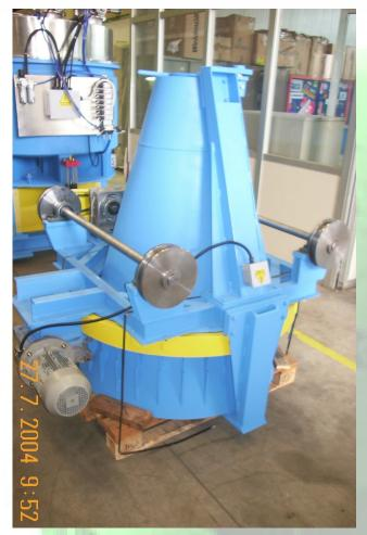
The paste distribution cone enables to collect the paste coming from the mixer and unload it in the pasting hopper.
