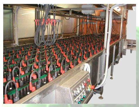
These charging containers are the best way to charge batteries. These water baths will be in plastic materials or in stainless steel, they are totally automatic either on the introduction of btr inside or on the download to the finishing line, on the opening and closing of the service doors, and on the fill/unfilling of the water.
