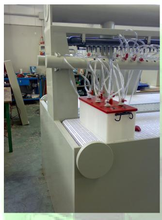
Module for the formation of truck battery with acid recirculation in a close loop cycle
