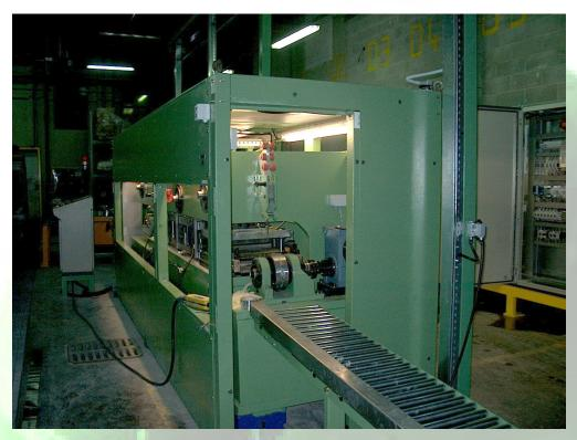
This is the heart of the Expanded Metal Line. completely NEW approach to **EX-MET** manufacturing. Through the use of 5 Electrical motors working together under mathematical algorithm, the achieves PERFECT expansion of the strip each and every time. Although the TITAN can run at speeds of upto 26 meters per minute, reliable, continuous and constant expansion is achieved at a speedof 23 m/min
