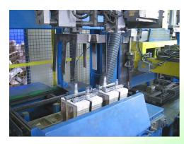
The correct tinning of the lugs, the right temperature of the pot feeding pipe and mould, allows the top quality strap production and the minimal dross production for a continuous high quality lead strap.
